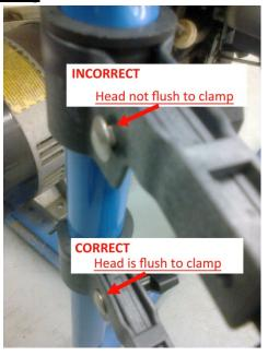
Please check to see that the carriage bolt is flush to the clamp before tightening! If you have already installed your GenTent, please double check that the carriage bolts are flush.
